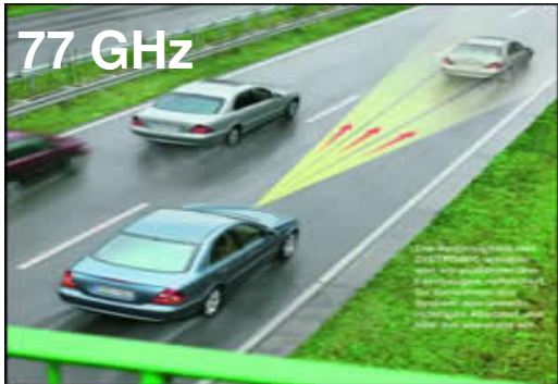
Adaptive cruise control radar for automobiles
